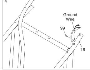
Loosen the two (one shown) Crossbar Screws (98) several turns. Place the Console Base (87) on the Right Handrail (16) and the Left Handrail (not shown). Make sure that the Wire Harness is not pinched in the Right Handrail. Attach the Console Base with four 3/4" Screws (43) (only two Screws are shown). Start all four 3/4" Screws before tightening them.
